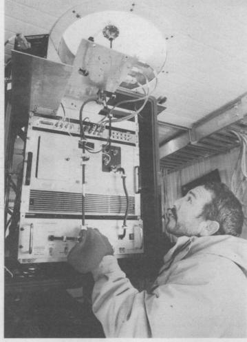
CLOUD WATCHER — Mark Aguilar (6612) makes adjustments to a cloud radar instrument in the Portable Arctic Atmospheric Radiation and Cloud Station — or PAARCS — during predeployment testing and integration at Sandia. The PAARCS will be stationed aboard an icebreaker in the Beaufort Sea north of Barrow, Alaska, for a 13-month drift amidst the arctic ice. (Photo by Mark Poulsen)
